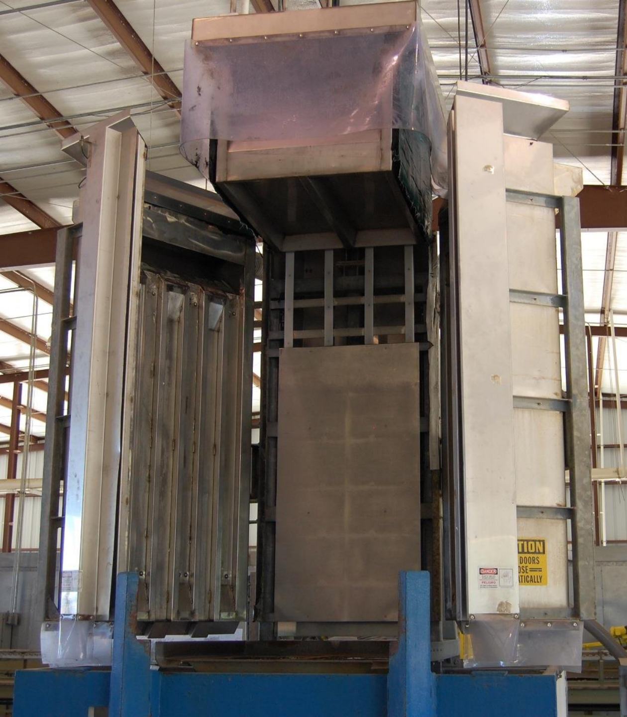
A “clamshell” type of package-icing cooler used for broccoli in Georgia
