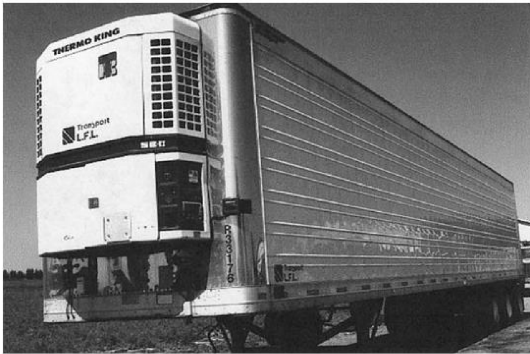
Fig. 3 Nose-mounted refrigeration system used in a semitrailer.
