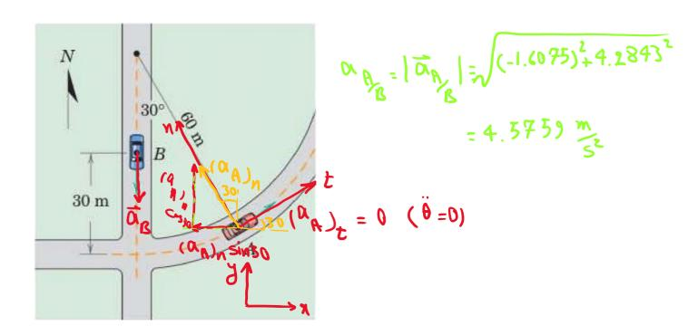
$$\overrightarrow{\alpha}_{B} = -1.5 \stackrel{?}{j} \frac{m}{s^{2}} \qquad \overrightarrow{\alpha}_{A} = -1.6075 \stackrel{?}{i} + 2.7843 \stackrel{?}{j} \qquad (\frac{m}{s^{2}})$$
