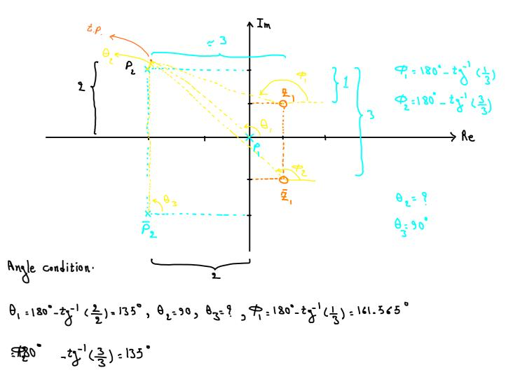
$$= \theta_{1} - \theta_{2} - \theta_{3} + \theta_{1} + \theta_{2} = \pm (2 \text{ k} - 1) |80^{\circ} = > -135^{\circ} - \theta_{2} - 90^{\circ} + 161.565^{\circ} + 135^{\circ} = \pm 180^{\circ} (2 \text{ k} - 1)$$
